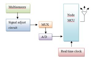
Fig. 2. Block diagram of Data Acquisition Module
