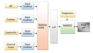
Fig. 1. Block diagram of the system
